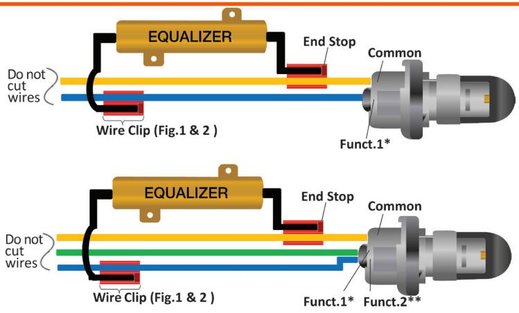
\*Funct. 1 - Wire not requiring load equalizer, such as parking/running light
