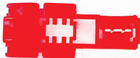
**4** Fold back the last part of the wire clip. This part has metal connectors that will push through the wire clip and cut through the two wires, connecting the current from the two. Ensure the clip is sealed tight with pliers. The wires should not be able to move around in the wire clip.
